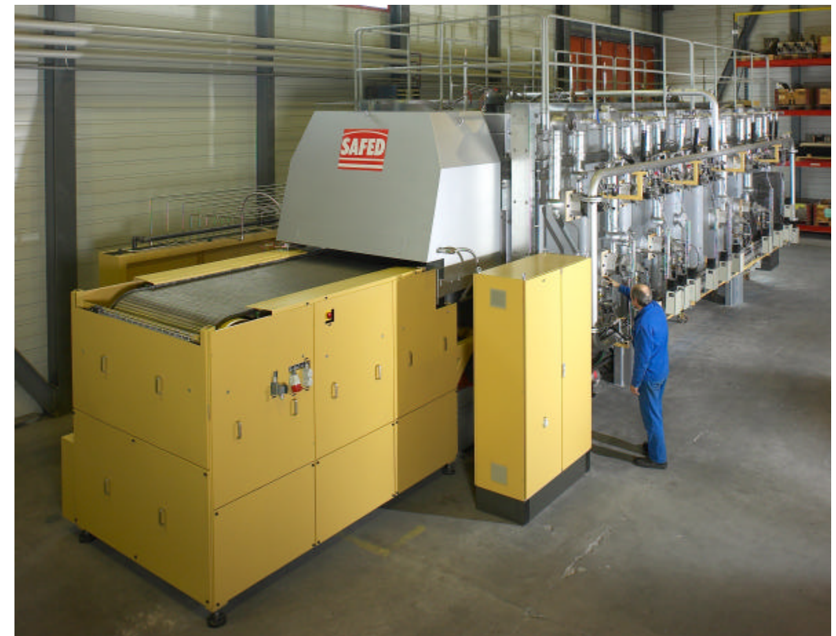
Type TC 160 furnace, gas-heated, capacity up to 1800 kg/h
