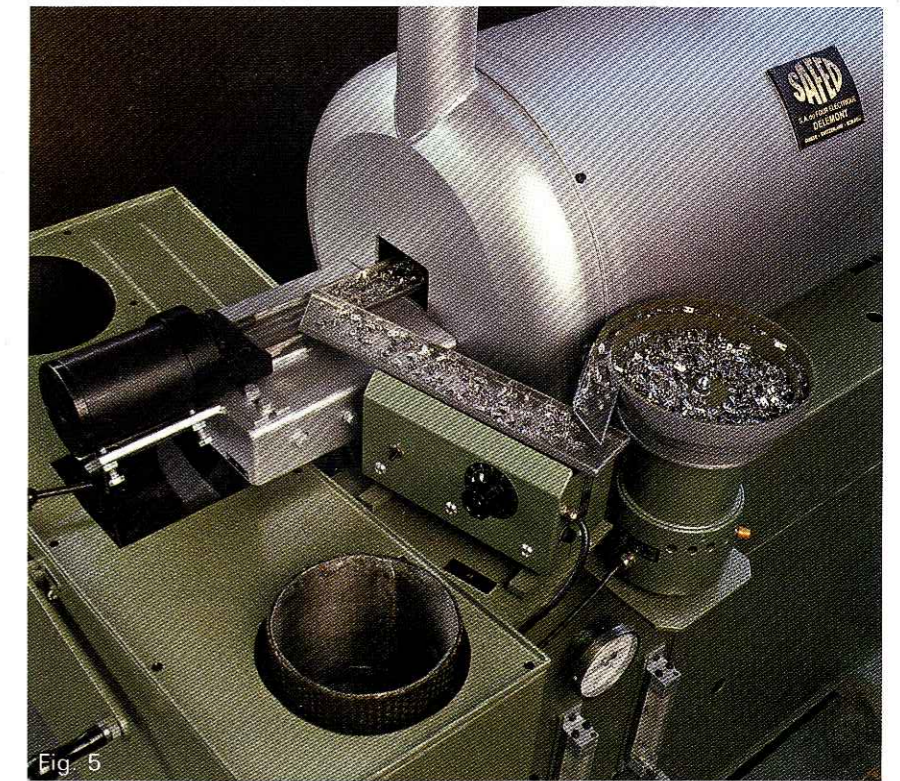
Fig. 5 Detail of automatic loading of shaker hearth furnace type Vi 9P.
