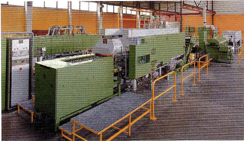
Fig. 6 Continuous heat treatment line for screws with automatic loader, mesh belt conveyor furnace type T 80/36 for carbonitriding, washing machine and furnace type 6 BdL 40/40 R for tempering with forced air circulation.
