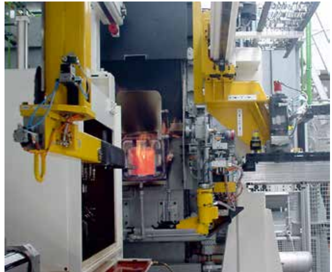
Rotary hardening of carburized TDI-camshafts with subsequent washing and tempering
