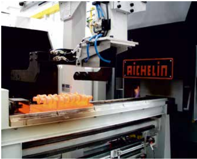
Carburizing and rotary hardening of shafts
