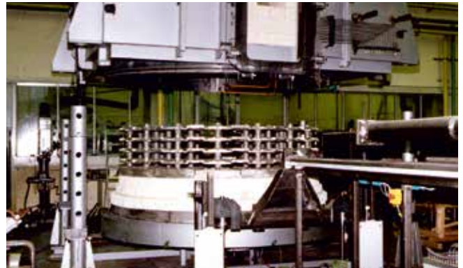
Final assembling multi-stage rotary hearth furnace
